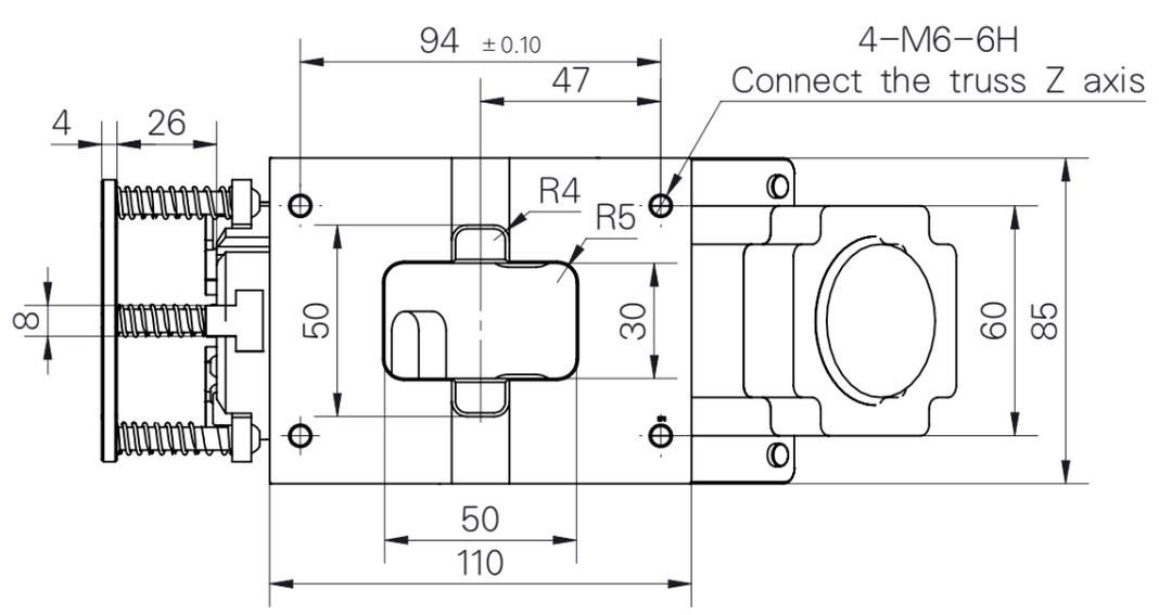
名称: 桁架三爪机械手 (Truss three-jaw manipulator)
